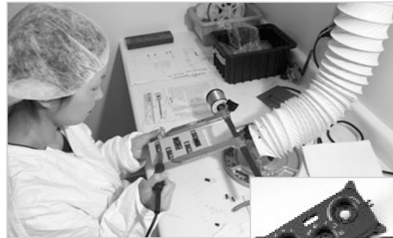
A Wilson-Hurd employee solders a circuit board in a "clean room" for use on a custom electronic control product. Inset: formed and molded IMD appliques for automotive dashboards.
