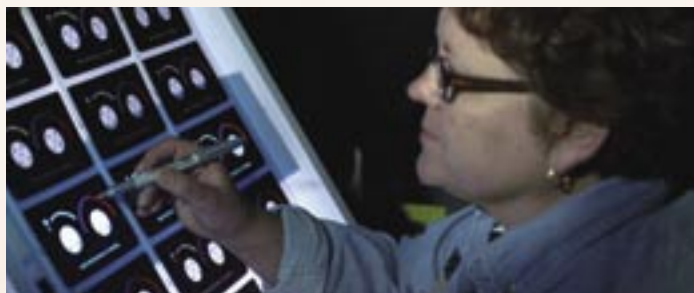
Light Booth for In-Mold Decorating (IMD) Inspection
